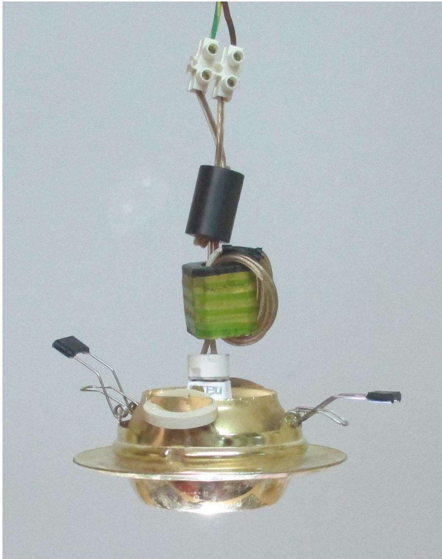
Figure 2 Domestic LED light with added filtering to suppress interference
