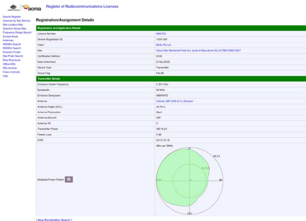
Figure 15: Image from ACMA site registration showing Ericsson AIR3239 radio hardware licenced at 295-degree sector bearing on 21 Apr 2021
