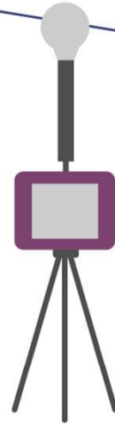
EME measurement probe positioned 1.5 m above ground at predicted maximum EME distance from base station
