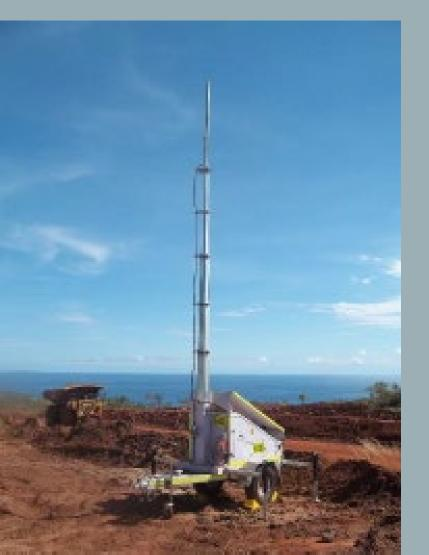
COWs currently restricted to 4W EIRPWiFi connectivity to satellite connected mobile base stations. Range limited to 400M using WiFi 6
