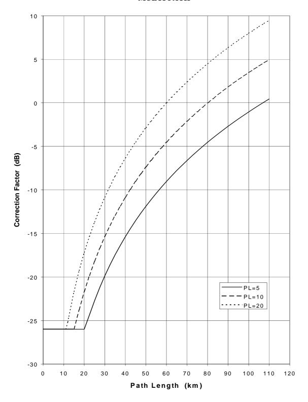
$P_L$ : Percentage of time that the average refractivity gradient in the lowest 100 m of the atmosphere is less than or equal to -100 N units/km.
